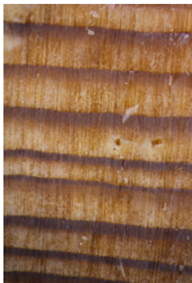
Figure XX. Transverse surface showing the abrupt boundaries between early and latewood cells, and the absence of resin ducts.
